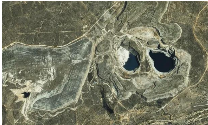
Fig. 6 – Pits of abandoned mine for PHS in Queensland, Australia. Photo: Genex
