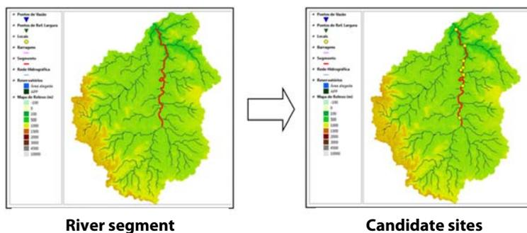
For each candidate site HERA evaluates the angle of the dam axis that minimizes the distance between the abutments identified from The DTM. The next step is to simulate the reservoir flooded area from the dam geometry with the DTM. Polygons are drawn and islands inside the reservoir considered in the final wet area and storage calculation. An optional buffer around the perimeter of the reservoir may be user defined to consider environment protection (as in many jurisdictions).
